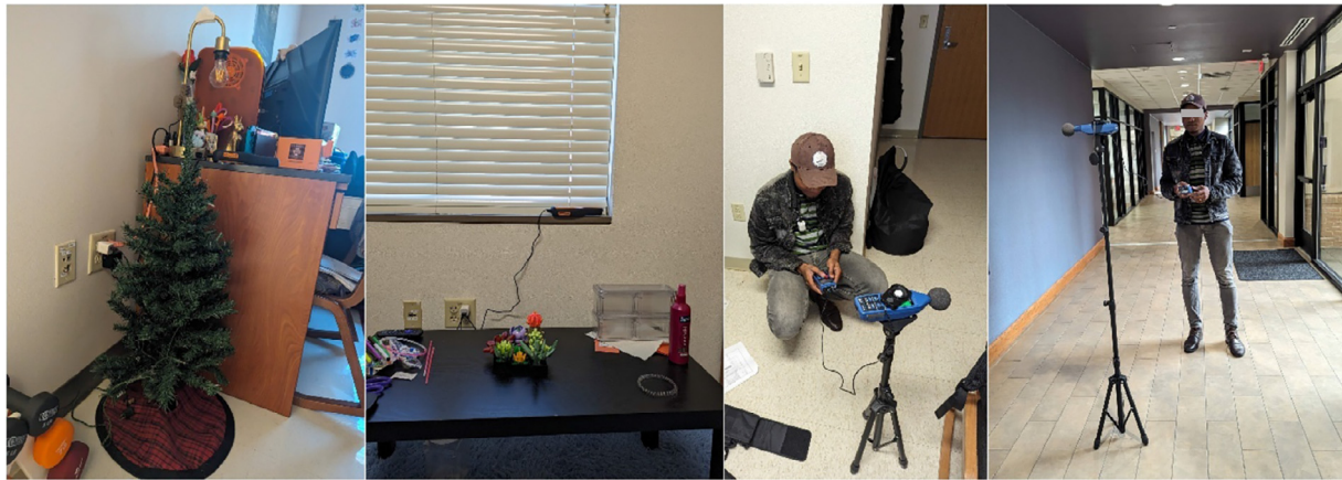
Fig. 3. Example field measurement setups for hygrothermal-IAQ (left two images) and lighting and acoustic assessments (right two images). The rightmost image depicts a corridor space, while the remaining images show dorm rooms.
